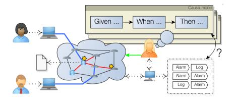
Scenario Networking / online collaboration Situation Impaired network service Observables Alarms and logs Diagnosis Situation understanding through causal models Real world Alarm spreading phenomenon, heterogeneous networks (multi-technology, multi-vendor)
